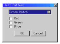
Press to display the test pattern. Pressing this button sequentially selects nine test patterns.
